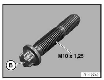
37. On vehicles from 12/12/2002 production, the M10 x 1.25 con rod bolts must be tighten at least **three** times in order to reach its maximum tensile strength.
