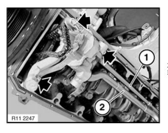
25. Remove oil pump return pipe (1) and suction pipe (2). Remove oil pump.
