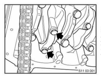
27. Connecting rod bearings bolts can be accessed from the bottom, in the following sequence: cylinders 1 and 6, cylinders 3 and 4, finally cylinders 2 and 5, when rotating crankshaft in clockwise direction. Using a special tool (p/n 90 88 6 115 100) at the crankshaft vibration damper pulley, turn crankshaft clockwise until number 1 cylinder connecting rod bolts are accessible.
