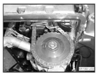
23. **Important:** To reduce tension exerted by the oil pump chain when loosening the sprocket nut, remove all slack existing in the chain. It can be done by tightening chain around the sprocket (as shown on the illustration) with approx. 7" of soft wire (e.g., from a wire hanger). This will protect plastic tensioner from possible damage while loosening the sprocket nut.
