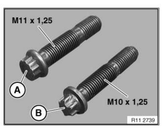
28. Remove connecting rod bolts (use M12 mm, 12-point socket on vehicles with M11 x 1.25 bolts; or Torx E12 on vehicles equipped with M10 x 1.25).
