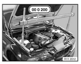
4. Install special tool (p/n 88 88 6 00 0 200 "engine brace") in engine compartment in order to support engine during the repair. For installation instructions refer to RA 11 13 000.
