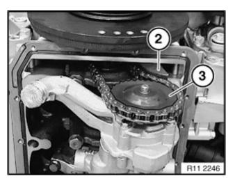
24. Press back the chain tensioner (2). Detach sprocket wheel (3) from oil pump shaft.
