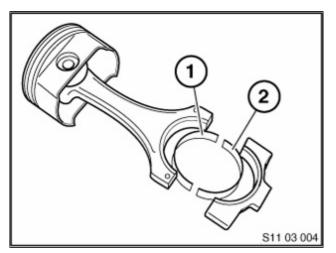
One classification of connecting rod bearings will be used in this Service Action. Connecting rod bearings are colorcoded:
