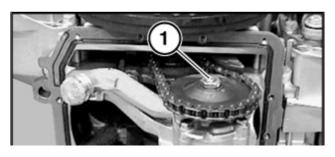
22. Using M17 mm socket remove oil pump sprocket nut (1).
