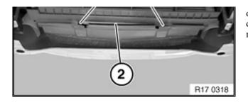
oil cooler (2) from the bottom of radiator without disconnecting oil hoses. Secure oil cooler to the body by means of plastic wire ties.
