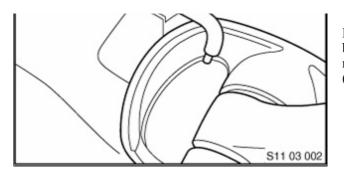
**Important:** When pulling down pistons for connecting rod bearing shell disassembly, make sure not to damage oil spray nozzles, which are located at the bottom side of the block (between crank bearing supports).
