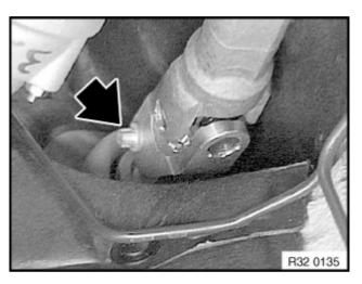
9. Detach steering spindle from the steering rack by removing clamping screw.
