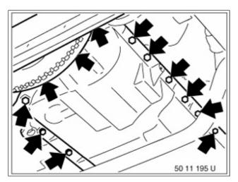
21. Unfasten oil sump screws and carefully remove oil pan.
